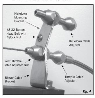
Step 6: Route kickdown cable housing up to the kickdown cable adjuster. If the cable housing is braided stainless steel, slide the ferrule back towards the transmission, away from the end that is being cut. DO NOT remove the ferrule from a braided stainless steel housing! If the housing is black universal, remove the ferrule. Add 1" extra and cut the kickdown cable housing to desired length. Make sure that the inner wire is removed from the cable housing before cutting!
